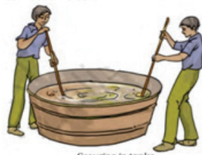
Scouring in tanks
